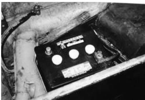
Step one in any electrical project, disconnect the battery. We'll donate this 6-volt to one of our antique car friends.
