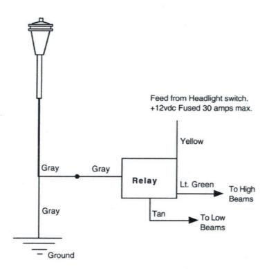
Tilt Lever (GM) with Switch and Relay for Hi/Lo Dimming
