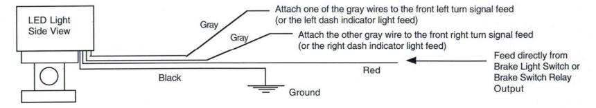
C. To have the center 30 LED's act as the 3rd brake light and the outer 15 LED's on each side work as turn signals AND as additional brake lights
