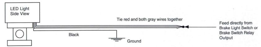
B. To have the center 30 LED's act as the 3rd brake light and the outer 15 LED's on each side work as turn signals ONLY
