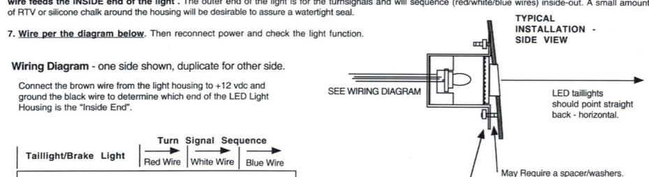
As a last step, add RTV or Silicone caulk to fill around the edge of the opening for a water tight seal.
