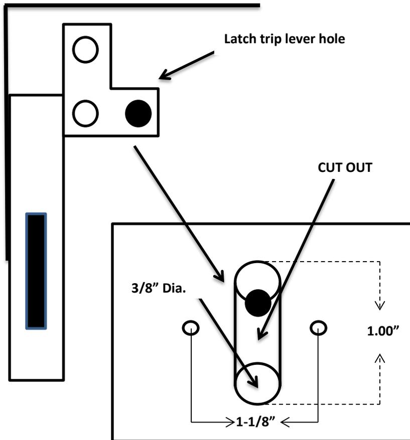
New holes shown in relation to the latch trip hole lever.
