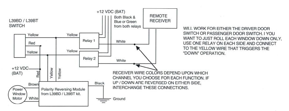
Alternative A8 - For Power trunk unit with a 5-wire switch, channels #3 - #4.
