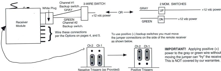
**IMPORTANT!** Applying positive (+) power to the gray or green wire without moving the jumper can "fry" the receiver. This is NOT covered by our warrantee.
