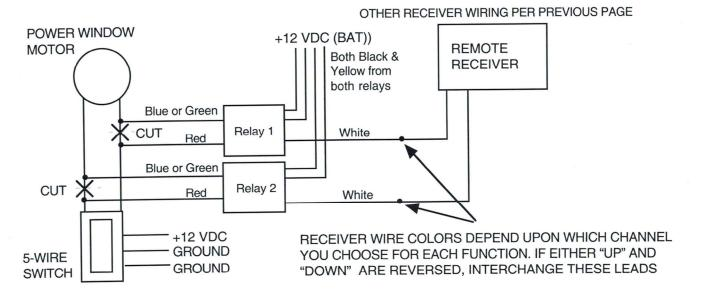
Alternative A4 - 2 door Power Windows DOWN ONLY with 5-wire switches. For only one door power window down, use only one side of diagram.
