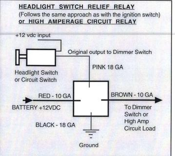
NOTE: Only the affected wires and connections of the Ignition Switch, Headlight Switch, etc. have been shown. For new circuit installation be sure to fuse both the switch hot (+) lead and the relay hot (+) lead according to the load being powered (the switch should be fused 2 - 5 amps max.).
