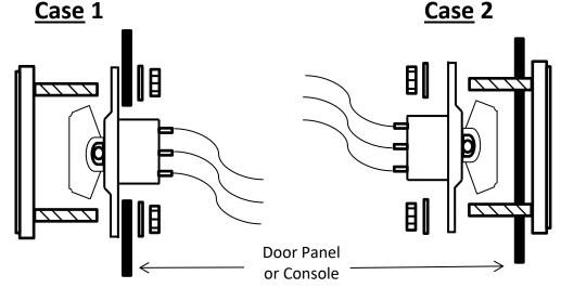
2. Cut Switch Holes using the template/ dimensions carefully mark and cut holes.
