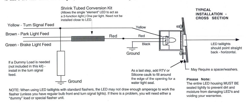
B. For vehicles that originally had integral brake/turn signal functions and are changing to separate brake/turn signal function - 40 LED's are RED brake and taillights, 12 LED's are AMBER turn signals.
