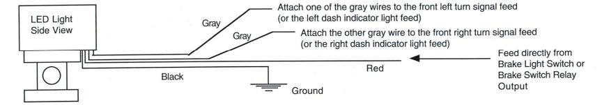
C. To have the center 30 LED's act as the 3rd brake light and the outer 15 LED's on each side work as turn signals AND as additional brake lights
