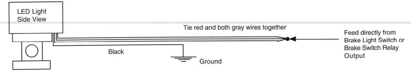
B. To have the center 30 LED's act as the 3rd brake light and the outer 15 LED's on each side work as turn signals ONLY
