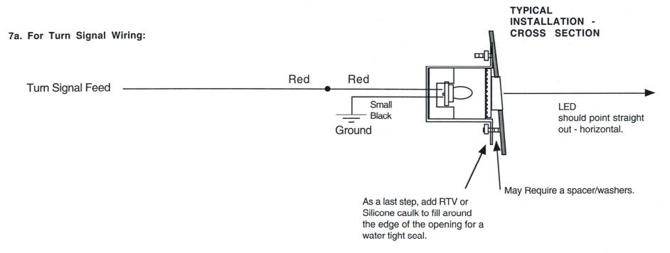
NOTE: When using LED lights for turn signals with standard flashers, the LED may not draw enough amperage to work the flasher (unless you have regular bulbs elsewhere in the system). If there is a problem with the flasher, you will need either a "dummy" load or special flasher unit.
