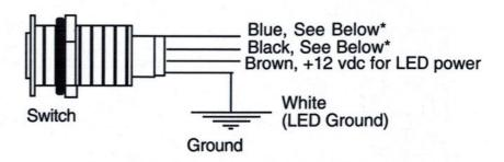
\* The Blue and Black wires are the ones controlled by the switch. They will be connected (continuous) when the switch button is pushed and disconnected when the switch button is released. They may be used to switch either positive or ground as your circuit needs. Also see the wiring diagram.
