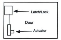
Typical Door Installation Use strap to install actuator and rod to connect to lock or latch release. StreetWorks also makes a cable connection kit with cable. pulley and hardware if that type connection would work better in your application.
