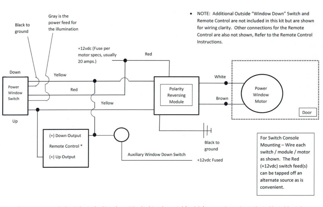
If you are mounting both switches in the driver door – Wire the driver door switch/module/motor as shown above. The Red (+12vdc) switch feed(s) can be tied together from the same source. The yellow switch wire leads off of the second (passenger door) switch must exit the driver door, crossover to and enter the passenger door and connect to the passenger door module/motor as shown.
